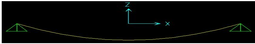
Figure 48. Span 2 deformed shape
