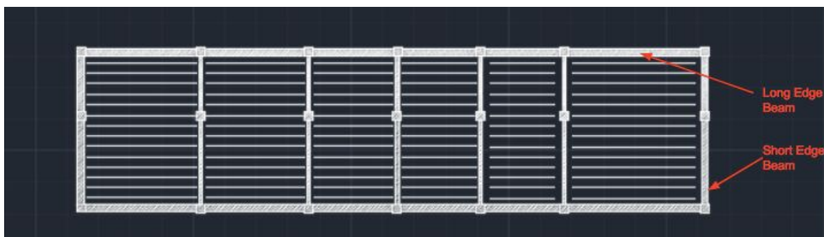
Figure 23. Exterior beams on office roof
